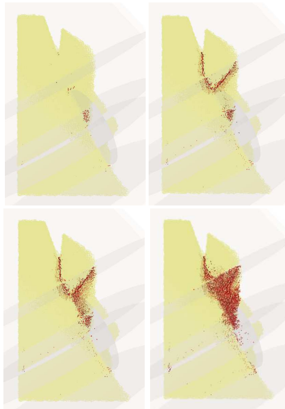
Figure 4. Vertical cut of the model. The set of discrete elements is in yellow. In grey, the discrete fractures and in red the cracks are represented. The upper left figure is plotted after 60,000 iterations, the upper right after 70,000 iterations, the lower left, after 80,000 iterations and the lower right after 120,000 iterations
