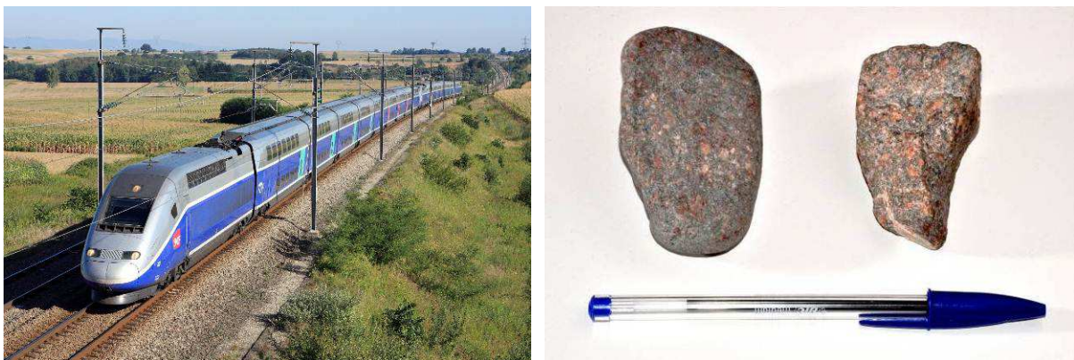
Figure 1. Left: TGV railway track lying over ballasted trackbed. Right: common samples of ballast grains (granite), around 6-7 cm long; the grain on the right is completely new (sharp edges), while the grain on the left has been eroded changing its morphology (rounded edges).
