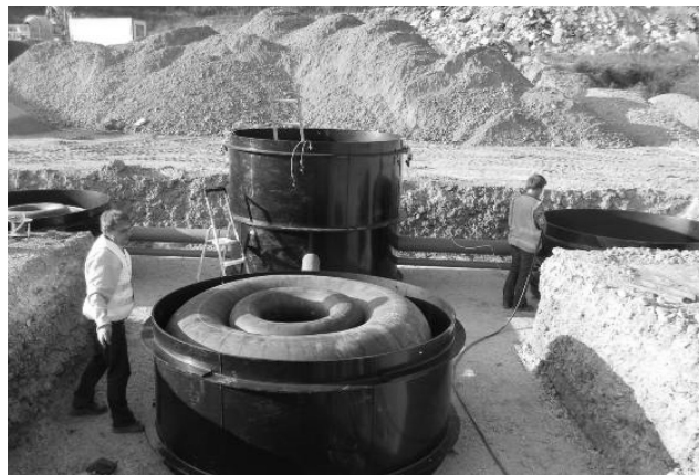
Figure 1. Installation of the experimental device for the progressive opening of a circular sinkhole under the geosynthetic-reinforced embankment
